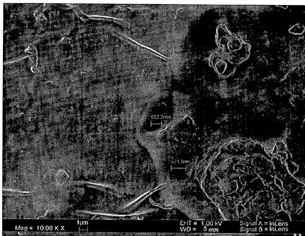
Figure 7. SEM picture of doped PANi film used in the PANi|AgCl set for doxycycline HCl diffusion
