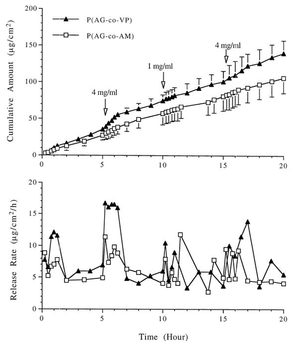
Fig. 7. Cumulative amount of the insulin released from erodible glucose-sensitive hydrogel matrices as a function of time. The hydrogels were prepared using PEGylated Con A (14 w/v%) and P(AG-co-AM) (2 w/v%) or P(AG-co-VP) (2 w/v%) ( $n=3$ ).
