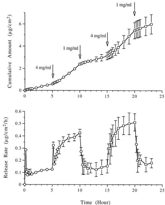
Fig. 3. Cumulative amount of the released insulin and insulin release rate as a function of time through glucose-sensitive hydrogel membranes under stepwise changes of the glucose concentration. The hydrogel was composed of PEGylated Con A (14 w/v%) and P(AG-co-SPAK) (3 w/v%). The glucose concentration at the receptor chamber was changed to either 1 mg/ml or 4 mg/ml at the times indicated by arrows ( $n=4$ ).
