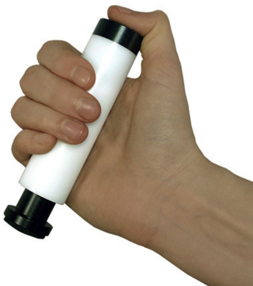
Fig. 3. D-Squame is a spring-loaded device that delivers the same amount of pressure every time on the D-Squame tape disc. The use of this device is not required, though it increases the consistency of the tape-stripping procedure. Image courtesy CuDerm Corporation.
