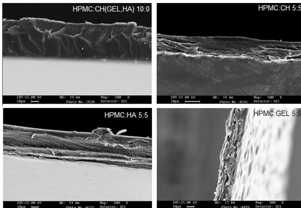
**Fig. 2.** Scanning electron micrographs of HPMC:CH(GEL,HA) 10:0, HPMC:CH 5:5, HPMC:HA 5:5 and HPMC:GEL 5:5 (scale bars: 10  $\mu\text{m}$  for HPMC:CH(GEL,HA) 10:0, HPMC:HA 5:5, HPMC:GEL 5:5; 20  $\mu\text{m}$  for HPMC:CH 5:5).
