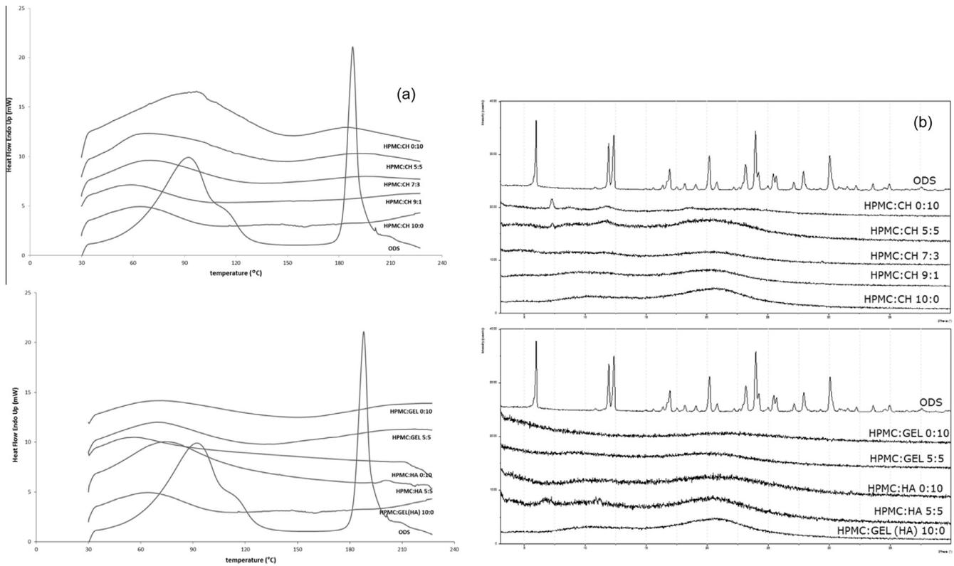
Fig. 3. Physicochemical characterization of buccal films: (a) DSC profiles of HPMC:CH (all the mixtures) and HPMC:HA(GEL) (all the most significant mixtures), with respect to pure ODS; (b) XRPD patterns of HPMC:CH (all the mixtures) and HPMC:HA(GEL) (all the most significant mixtures), with respect to pure ODS.
