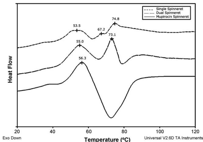
**Fig. 6.** DSC thermograms of mupirocin only (—) showing no drug crystallization, DS fiber scaffold (---) with no mupirocin crystals, and SS fiber scaffold (· · ·) indicating lidocaine hydrochloride and mupirocin crystallization in the polymer domains.
