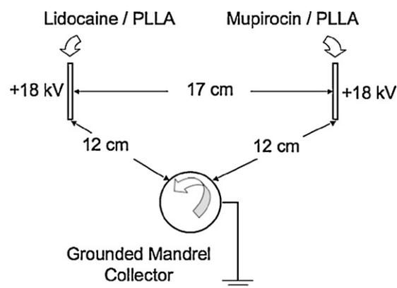
Fig. 1. Schematic of the dual spinneret electrospinning apparatus.
