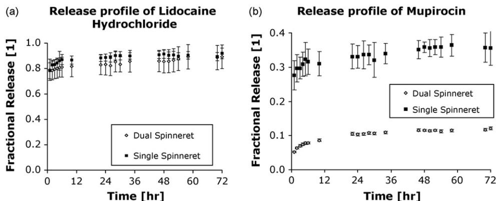
**Fig. 5.** Release profiles of lidocaine hydrochloride and mupirocin incorporated in PLLA and electrospun by the DS or SS technique. (a) LH eluted from DS (◆) and SS (■) scaffolds demonstrate a burst release followed by a plateau. (b) Mupirocin eluted from DS (◆) and SS (■) scaffolds demonstrate different magnitudes of burst release followed by a slow release. Error bars indicate 95% confidence interval,  $n = 5$ .
