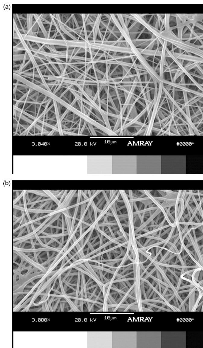
**Fig. 3.** SEM images of (a) DS electrospun scaffold and (b) SS electrospun scaffold.
