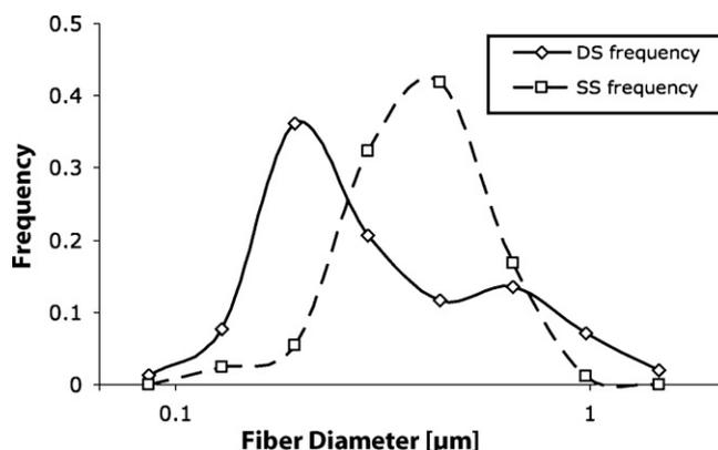
**Fig. 4.** Distribution of fiber diameter in dual-spinneret scaffold versus single spinneret scaffold, note the use of a logarithmic axis.
