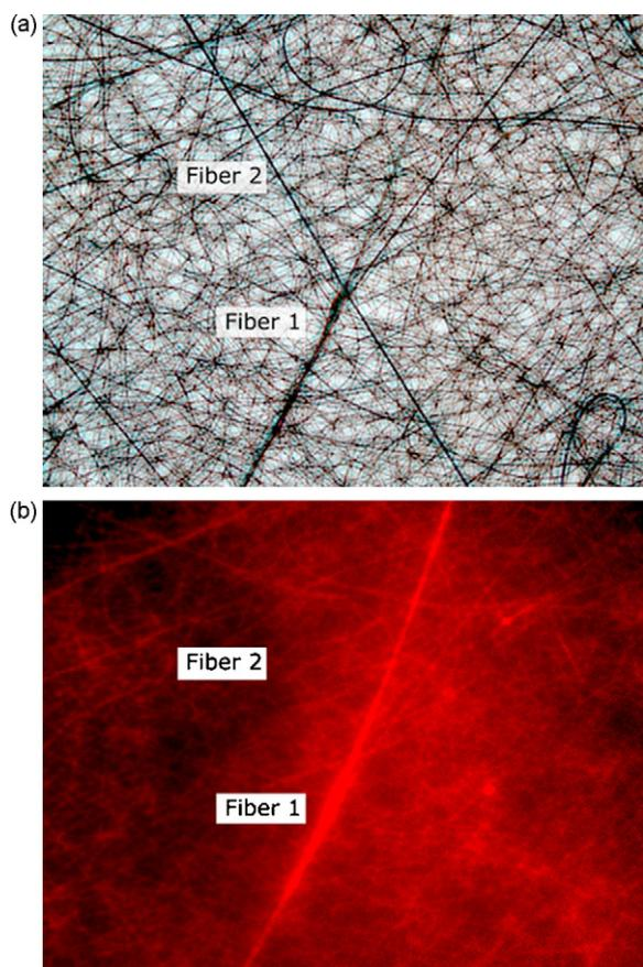
**Fig. 2.** Light microscopy (a) and fluorescence (b) images of electrospun fiber scaffolds fabricated by DS technique. Fiber 1 is clearly visible by both imaging techniques, while fiber 2 is not visible by fluorescence microscopy.
