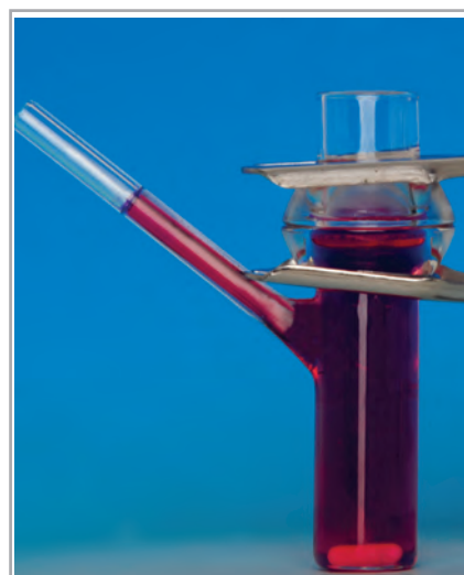
Fig. 4 Franz Diffusion Cell. Images courtesy of Mr. Pütz, Saarland University
