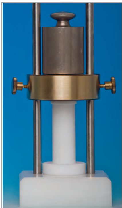
Fig. 7a Saarbrücken penetration model from the front. Images courtesy of Mr. Pütz, Saarland University
