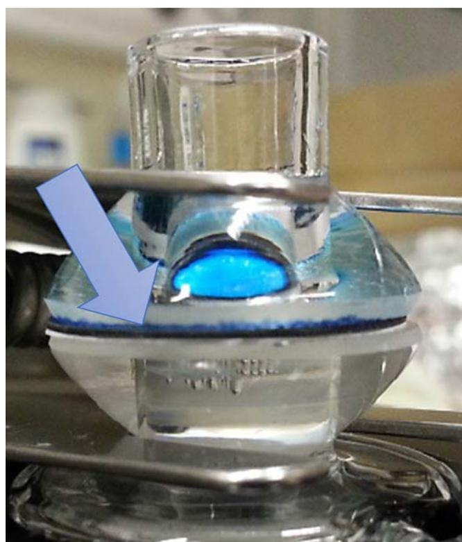
**Fig. 2.** Using seal No. 2 (sheet gasket), the lotion formulation dispersed widely outside the application zone (arrow).
