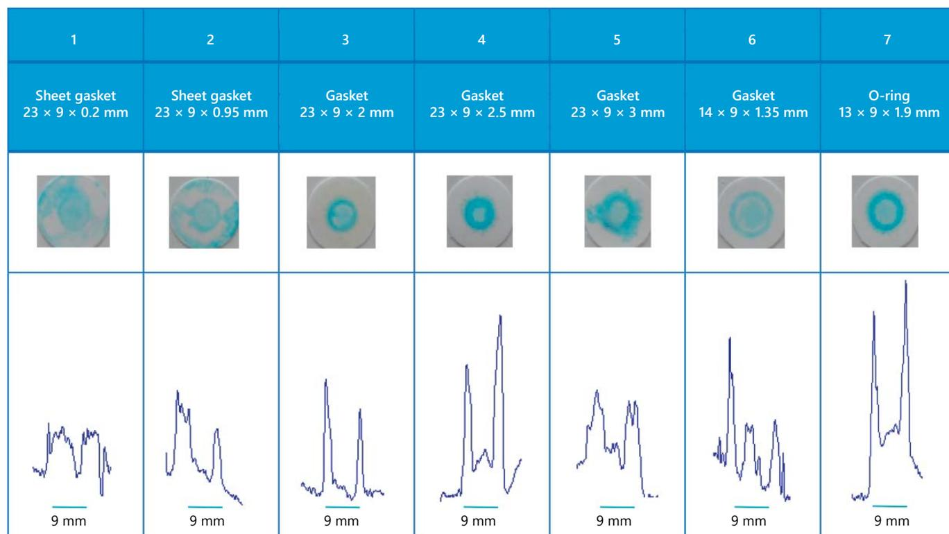
**Fig. 3.** Visual result and VIS profile of seven different seals used in an FDC system for measuring the in vitro dermal absorption.
