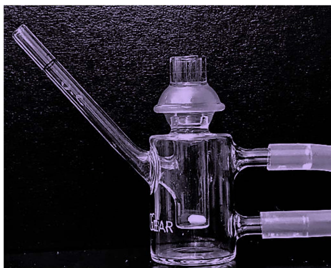
Fig. 2. Photographic image of spherical joint Franz diffusion cells used for transcorneal permeation studies.
