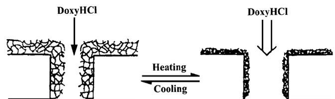
**Fig. 6.** Thermo-sensitive permeation of doxycycline HCl through polymeric gel-immobilized PVDF membrane (adapted from [8]).
