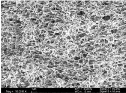
(b) Cross section image of PNIPAAm-PVDF membrane
