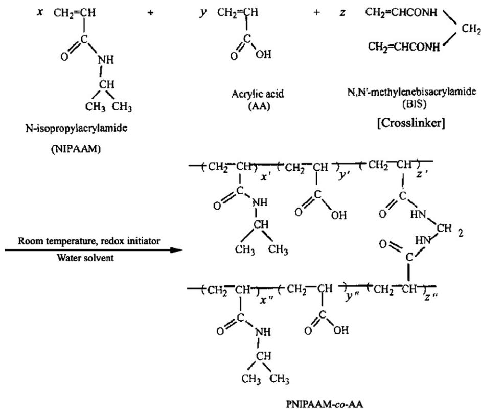
Fig. 1. Schematic of PNIPAAM-co-AA synthesis (modified from ref. [13]).
