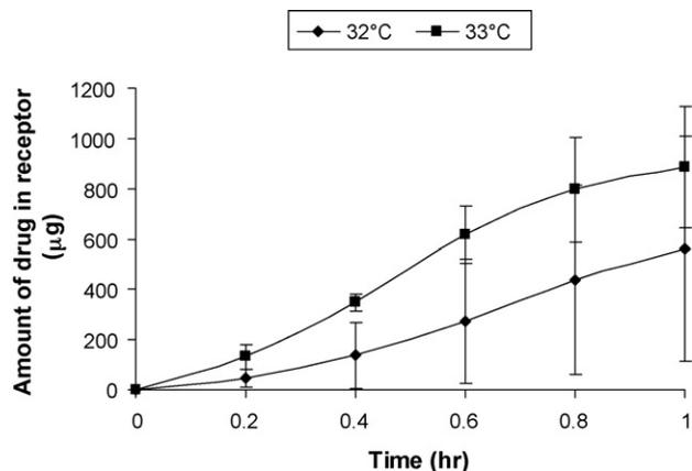
**Fig. 3.** *In vitro* release of doxycycline HCl using light mineral oil as vehicle through 2%AA-PVDF membrane at two temperatures over 1 h.
