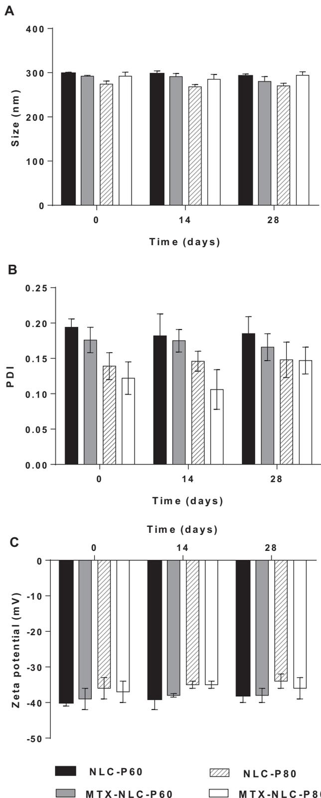
**Fig. 1.** Storage stability. Effect of time of storage at 25 °C on particle size (A), PDI (B) and zeta potential (C) of void and MTX-loaded NLCs. All data represent the mean ± standard deviation ( $n = 4$ ). No statistically significant differences were observed over the time for any formulation ( $P > 0.05$ ).
