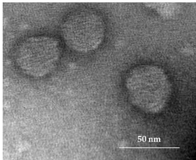
**Fig. 2.** TEM microphotograph of mixed micelles at ×400,000
