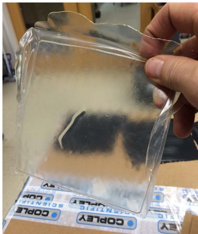
Fig. 2. Thermoplastic 80A polyurethane elastomer film use to create non-irritant polymer samples.
