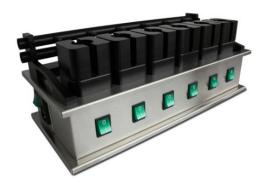
Jacketing the diffusion cells refers to the presence of a water jacket. The water jacket is typically connected, either directly or indirectly, to a circulating water bath which will maintain the membrane temperature at 32 °C or 37 °C depending on the test requirements. Unjacketed cells can have temperature control if the end user is able to immerse them in a waterbath or place them into an incubator.
