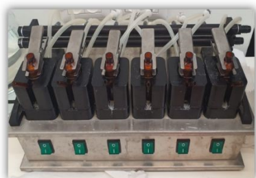
Scheme 1. Efficacy experiments with a Franz diffusion cell apparatus image (PermeGear, PA, USA).
