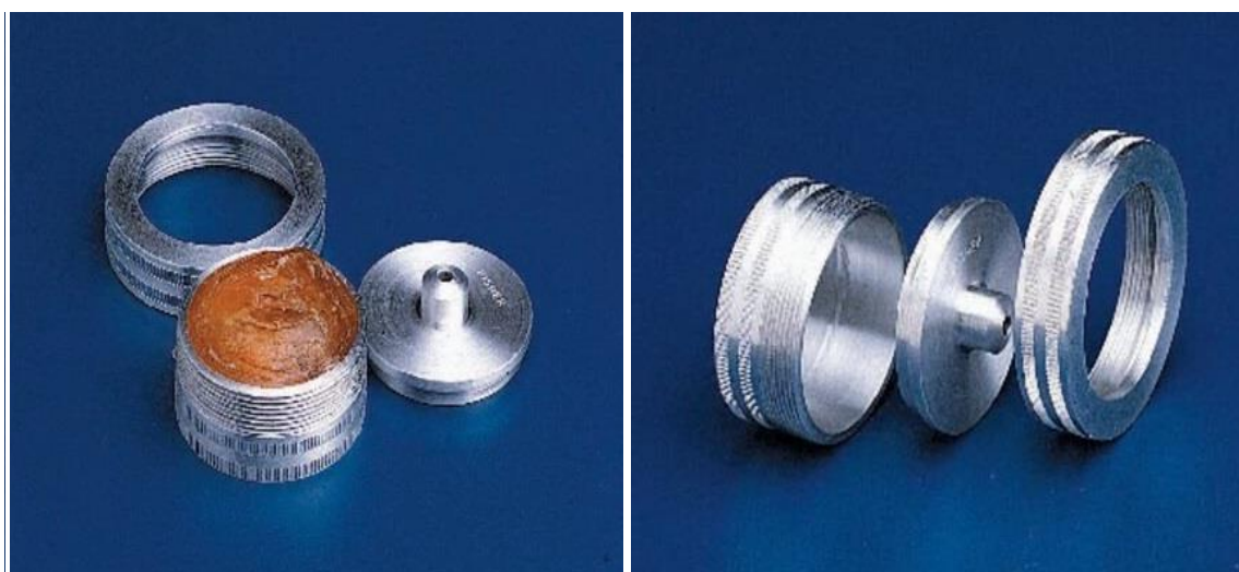
Figure 4.2. Photographs of specific gravity measurement device - stainless steel pycnometer [21].
