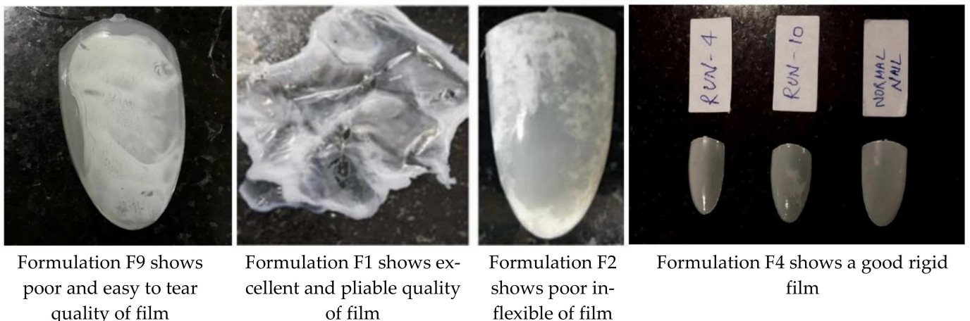
Figure 2. Various qualities of films obtained during optimization of nail lacquer with different ratios of solvents (Ethanol: Water) and polymers (HPC: Eudragit RS).
