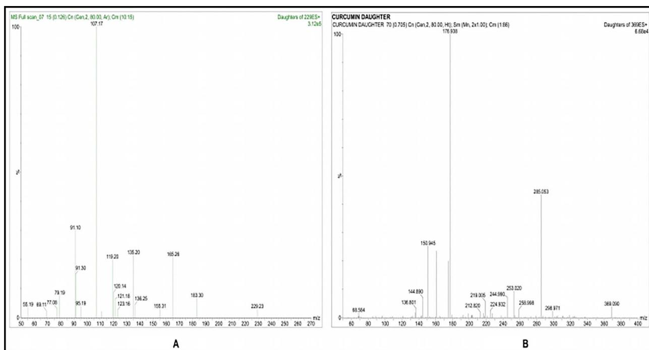
**Figure 3.** Chromatograms achieved following MRM of (A) RV as pure drug and (B) CUR as IS.
