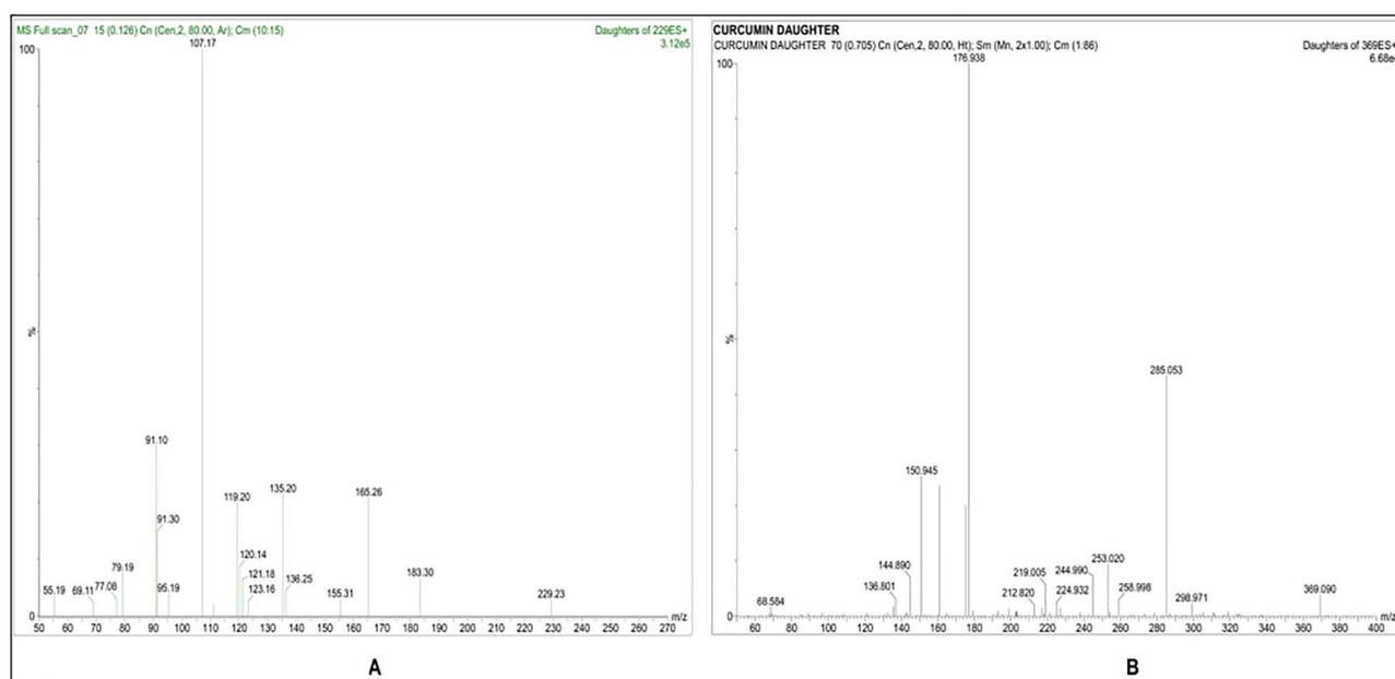
**Figure 2.** The daughter ion  $[M + H]^+$  ion spectra are illustrated by (A) RV (molecular weight 107.17) and (B) CUR (molecular weight 176.93) as in the positive ion mode.
