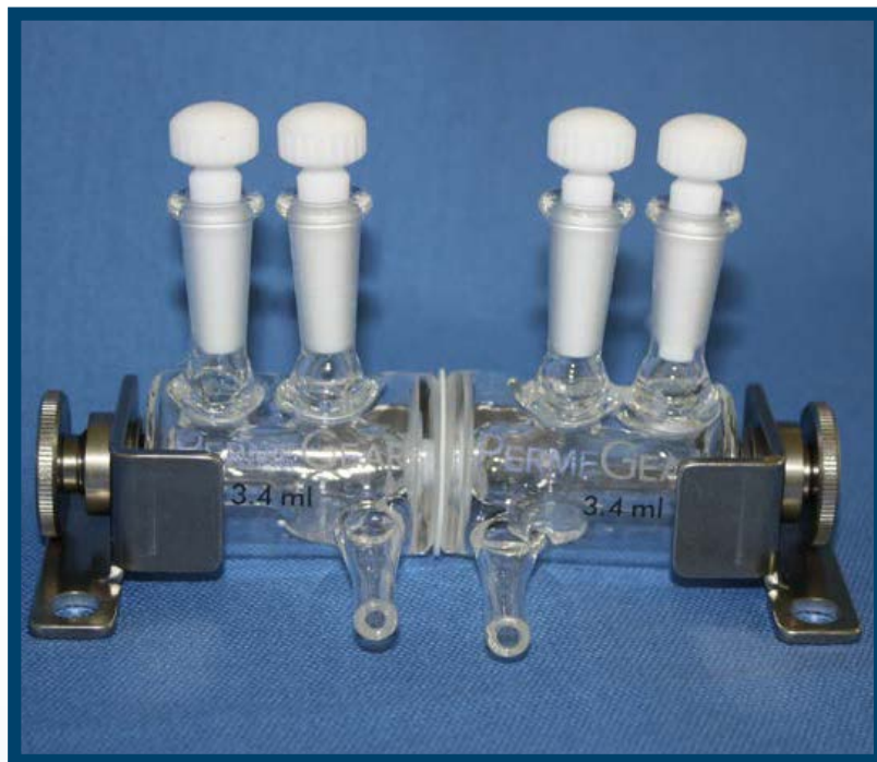
This Side-Bi-Side Cell has the common 9mm orifice diameter with 3.4ml standard volumes.
