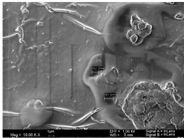
Fig. 8. SEM picture of doped PANi film used in the PANi|AgCl set for doxycycline HCl diffusion showing no white-gel-like precipitation layer to block the pathway of doxycycline HCl transportation.
